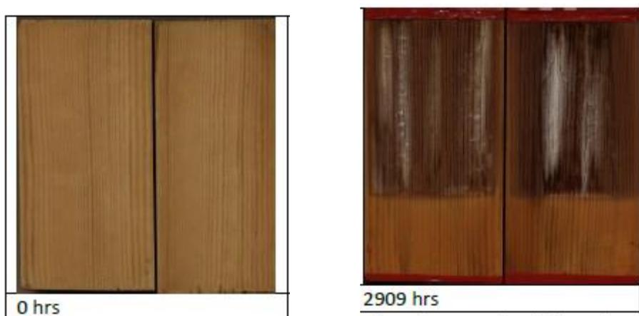
Figure 3: Non-stabilized alkyd formulation before and after 2,909 hours of exposure
