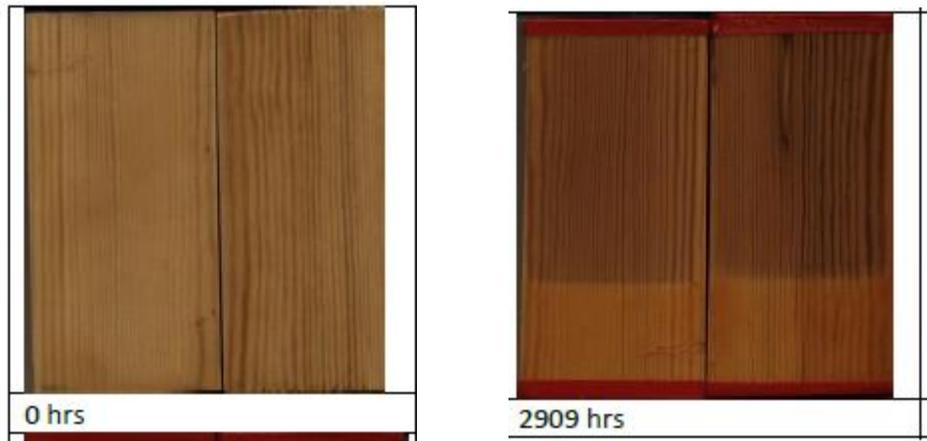
*Figure 4: Stabilized alkyd formulation before and after 2,909 hours of exposure*
