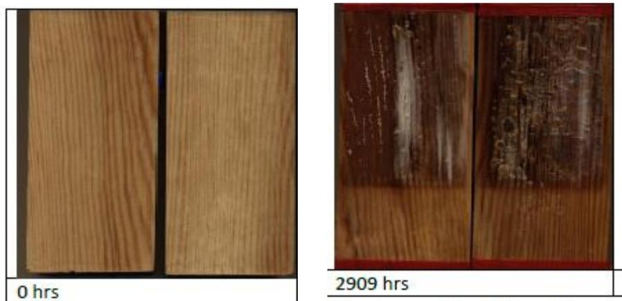
*Figure 5: Non-stabilized PUR formulation before and after 2,909 hours of exposure*
