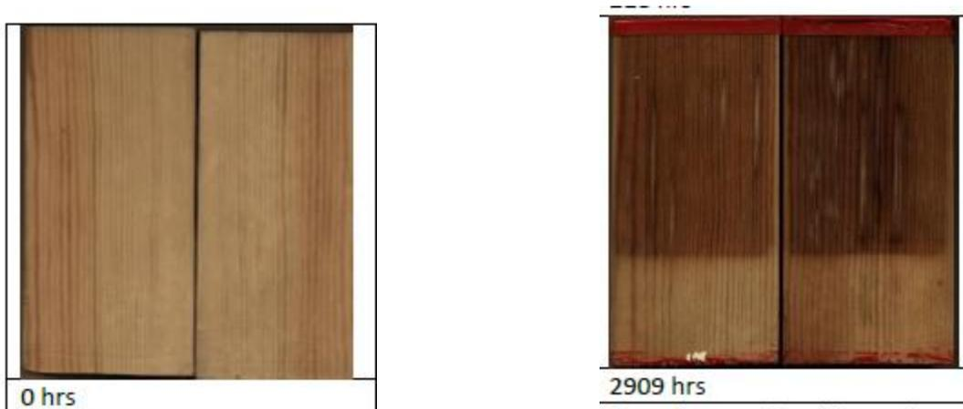
Figure 2: Formulation stabilized with SONGSORB® CS 400 WB and a HALS before and after 2,909 hours of exposure
