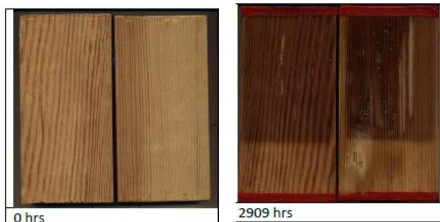
*Figure 6: Stabilized PUR formulation before and after 2,909 hours of exposure*
