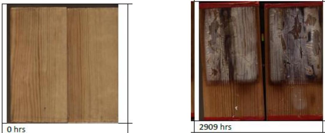
Figure 1: Non-stabilized acrylic formulation (no UVA and no HALS) before and after 2,909 hours of exposure
