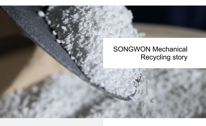
SONGWON supports the mechanical recycling industry with antioxidants for re-stabilization of recycled polyolefins.
